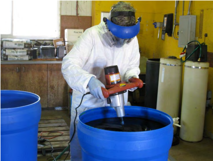
Figure 4-5: Mixing fluorescein in 55 gal. drums.
