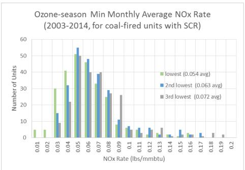
Figure 1. "Frequency" distribution plots for 272 coal-fired units with an SCR showing their  $NO_x$  emission rates (lbs/MMBtu) during ozone seasons from 2003-2014. For each unit, the best, second best, and third best ozone-season average  $NO_x$  rate (top panel) and minimum monthly average  $NO_x$  rate (bottom panel) are illustrated.
