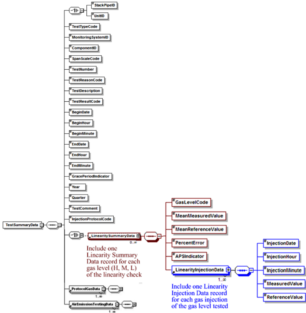
Figure 9: Linearity Checks XML Structure (Including: Test Summary Data, Linearity Summary Data, and Linearity Injection Data)
