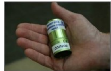
The CairClip air sensor fits in the palm of a hand and collects data on ozone and nitrogen dioxide in the air.
