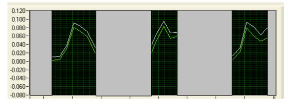
WHITE: Sample spectrum (minus H2O) GREEN: 150ppm NO calibration spectrum
