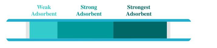
Desorb the tube in the direction of strong adsorbent to weak adsorbent
