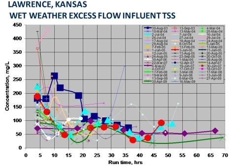
First-flush dynamics are much different than conventional POTW diurnal design and operation standards
