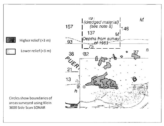
Figure 2. Hard bottom features having significant vertical relief outside Arecibo Harbor. Based on EPA Region 2 side scan SONAR survey (conducted November 2011)
