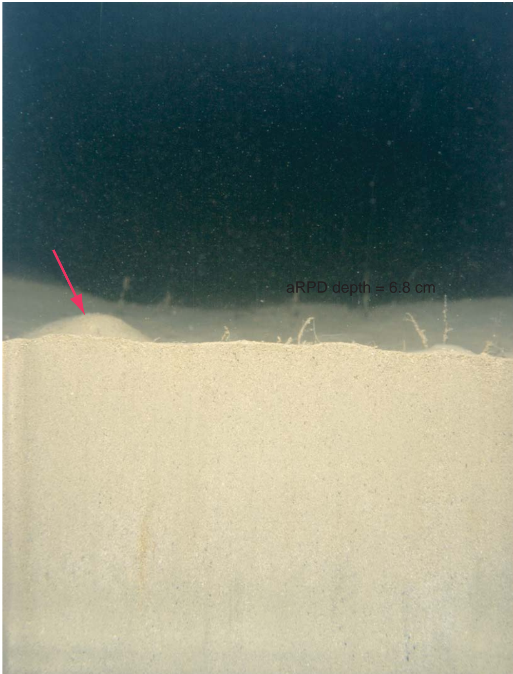
Figure 3-9: In this SPI image from station F8, the small-scale vertical relief across the field-of-view (i.e., "boundary roughness") is due both to sediment accumulation around the upright tubes and to the biogenic mound at left (arrow). This is an example of biogenic boundary roughness. Scale: actual image width is 14.4 cm.
