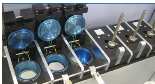
Figure 5. Photo of micro-chamber/thermal extractor ( \mu CTE) from Markes International, Llantrisant, UK (Cleanroom Technology, 2011)
