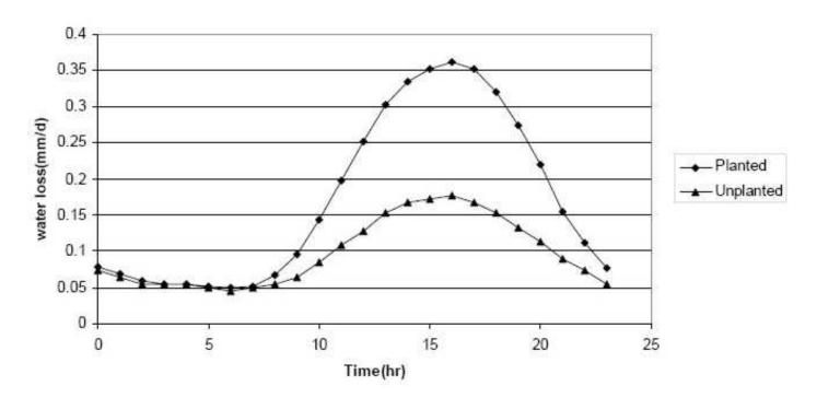
Figure 5-3 Average hourly water loss from planted and unplanted boxes for the 2nd day after watering during the hot summer condition (Rezaei 2005)
