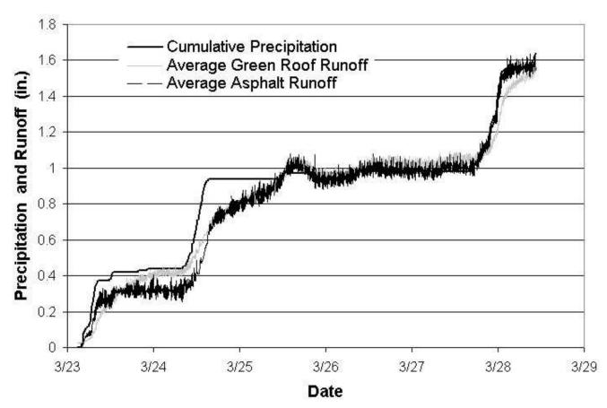
Figure 3-6 Precipitation and green and asphalt roof runoff from snow and mixed precipitation events in March, 2005
