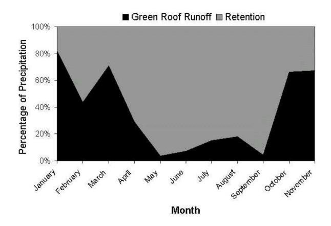
Figure 3-1 Retention and runoff from green roofs (percentage of average monthly precipitation)
