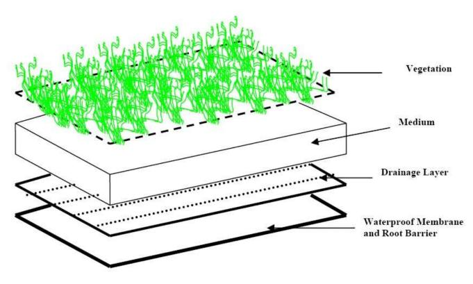
Figure 1-1 Typical cross-section of a green roof system (Berghage et al., 2007)
