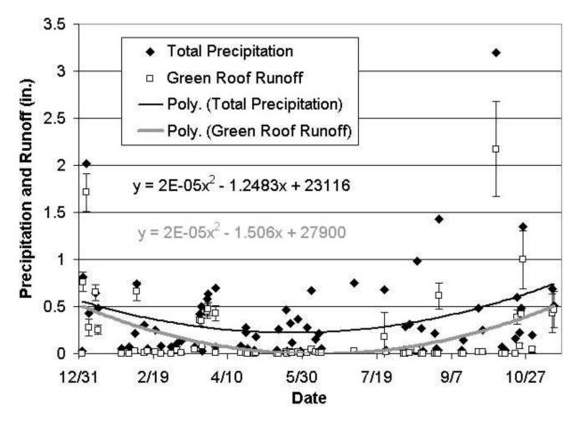
Figure 3-4 Plot of precipitation versus runoff from green roofs for paired events
