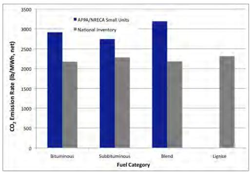
Figure 3-6. CO2 Emission Rates for Small EGUs vs. National Inventory, By Coal Rank
