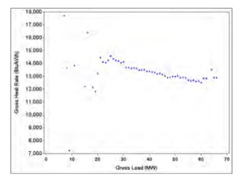
Figure A-1. Gross Plant Heat Rate vs. Load: CR Lowman Unit 1
