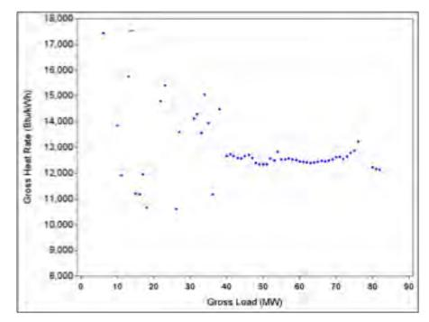
Figure A-2. Gross Plant Heat Rate vs. Load: Muscatine 8
