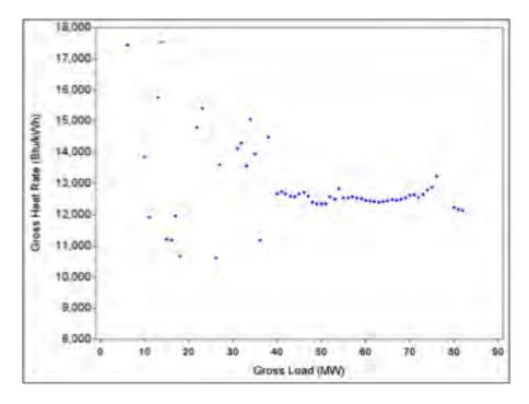
Figure A-2. Gross Plant Heat Rate vs. Load: Muscatine 8
