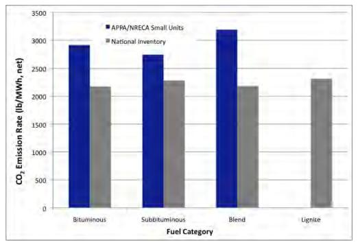
Figure 3-6. CO<sub>2</sub> Emission Rates for Small EGUs vs. National Inventory, By Coal Rank
