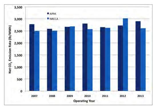
Figure 3-2. CO2 Emission Rate (Net) for Small APPA/NRECA EGUs, 2007-2013
