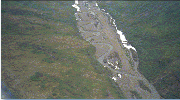
Figure 3. Caribou Creek in 2002 after NPS leveled and contoured large tailings piles to restore natural channel meanders and riparian function.
