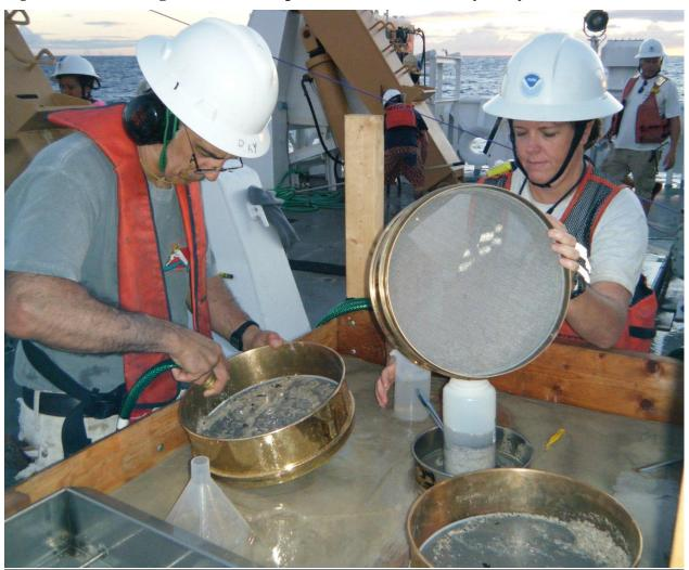
Figure 12. Processing a sediment sample for benthic community analysis.
