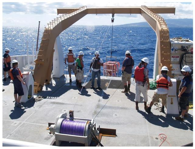
Figure 4. SPI-PVP camera system being deployed from the Hi'ialakai.
