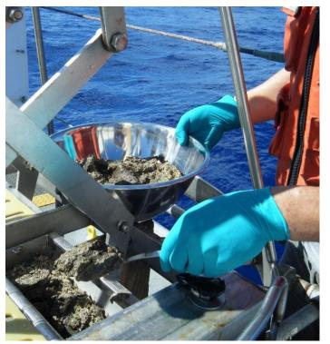
Figure 10. Subsampling from the Van Veen grab for sediment chemistry.
