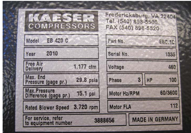
Kaeser blower label, indicating product was made in Germany. (EPA OIG photo)
