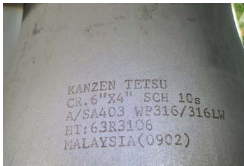
Pipe at the Ottawa project site labeled as made in Malaysia ( left ) and China. (EPA OIG photo)
