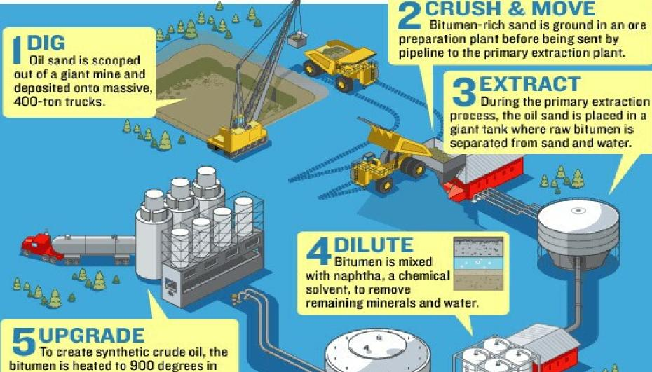
bitumen is heated to 900 degrees in giant furnaces, a process that removes excess carbon. Hydrogen is added to prepare it for industrial use.
