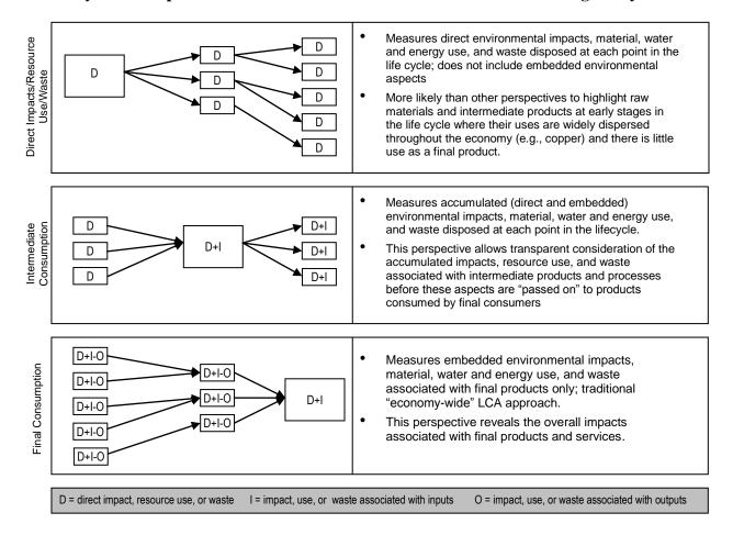
Figure 1 System Perspectives Considered in the 2020 Vision Relative Ranking Analysis
