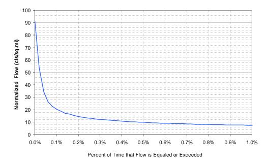
Figure 5: High flow portion of the Potash Brook flow duration curve.
