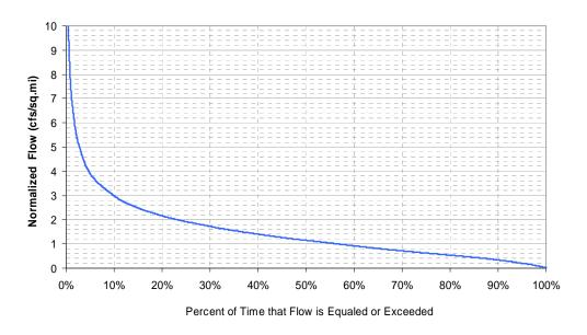
Figure 4: Potash Brook flow duration curve.
