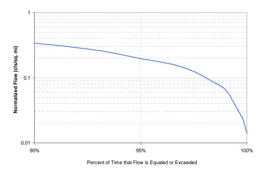
**Figure 6:** Low flow portion of the Potash Brook flow duration curve
