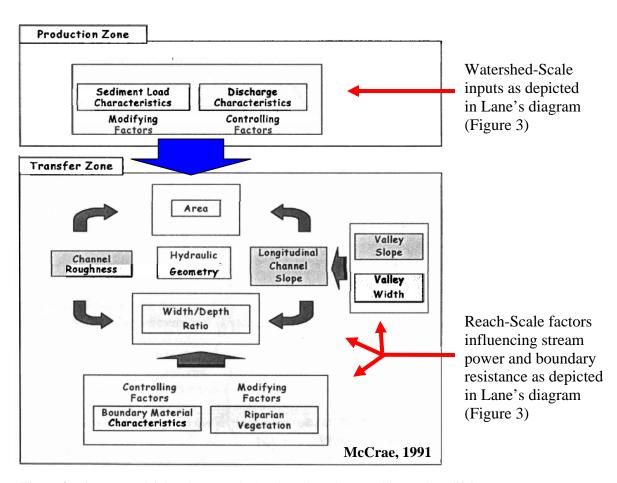
**Figure 2.** Diagram explaining the watershed and reach-scale controlling and modifying factors affecting the hydraulic geometry and fluvial processes of a stream.
