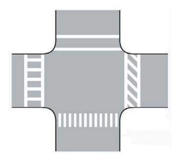
Typical standards require that crosswalks be composed of solid white lines, 6 to 24" wide. The width of the crosswalk should be a minimum of 6". The city of Detroit or Michigan Department of Transportation will dictate local crosswalk standards. The following layouts are most commonly used for crosswalks:
