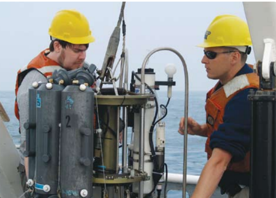
◀ CT DEP staff deploy a rosette, a water sampling device, aboard the research vessel John Dempsey .
