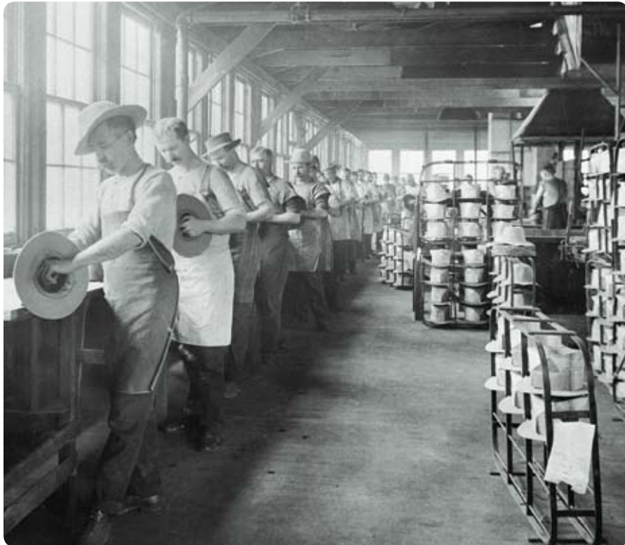
◀ Workers finishing hats in the early 20th century at a factory in Danbury, CT, once the hatmaking capital of the world. Many workers were poisoned by long-time exposure to mercury used in the felting process.
