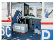
An Airborne Real-Time Cueing Hyperspectral Enhanced Reconnaissance sensor. (U.S. Geological Survey photo)
