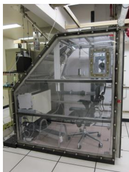
An EPA human subjects air pollution test chamber. (EPA OIG photo)
