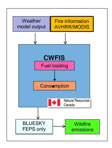
Figure 2: A functional diagram of the FireWork components
