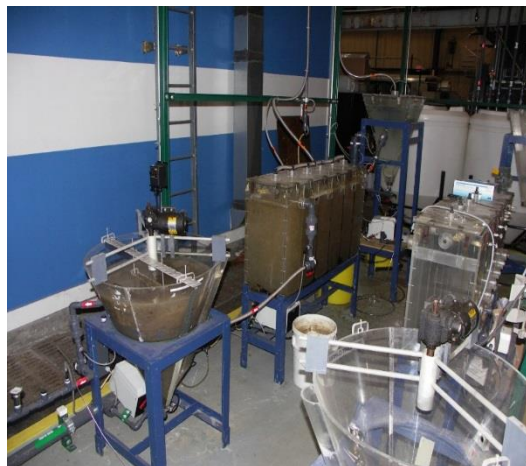
Pilot-scale facility for contaminant fate through waste water treatment, especially activated sludge. systems
