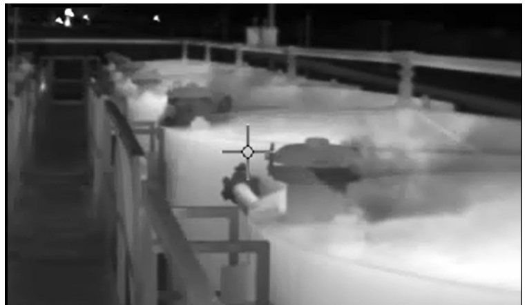
Infrared video image of thief hatch emissions.
