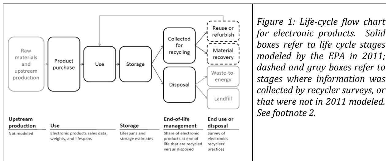
*Figure 1: Life-cycle flow chart for electronic products. Solid boxes refer to life cycle stages modeled by the EPA in 2011; dashed and gray boxes refer to stages where information was collected by recycler surveys, or that were not in 2011 modeled. See footnote 2.*
