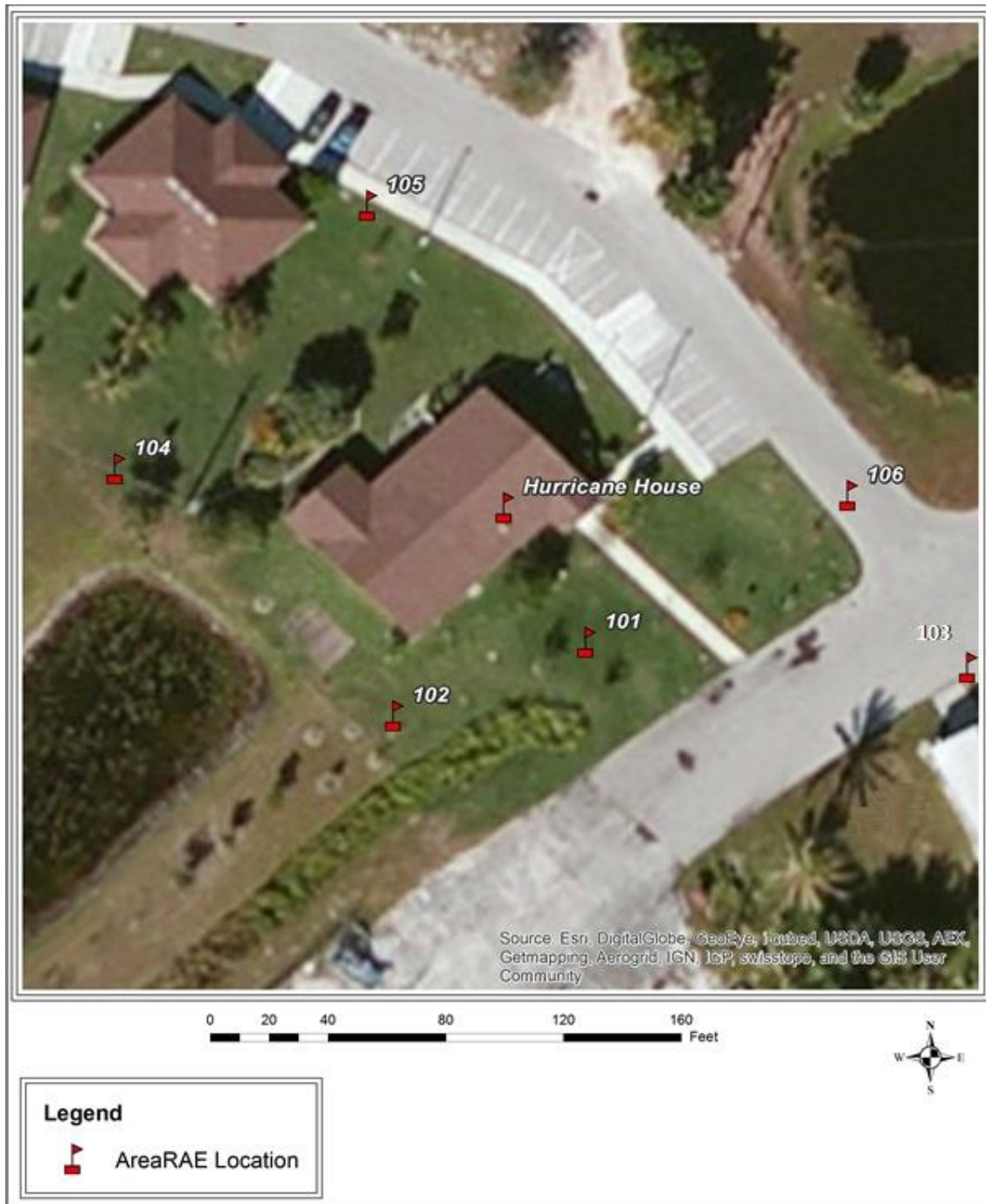
Figure 23. Ambient Air Monitoring Locations.
