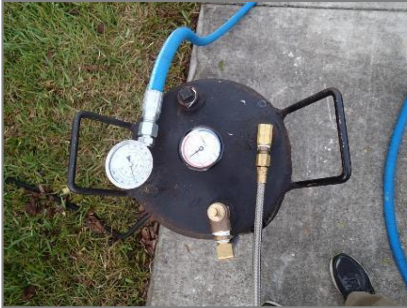
Figure 27. Heat Exchanger Used to Convert Liquid MB to Gaseous MB Exiting the Blue Shooting Hose
