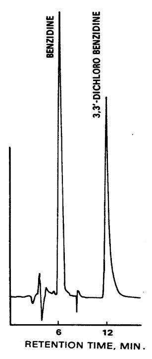
Figure 1. Liquid chromatogram of benzidines.
