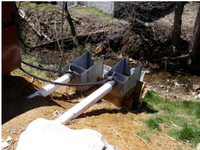
Figure C-12. Underdrains from permeable pavement equipped with 30-degree V-notch weir boxes and samplers for flow and water quality monitoring.
