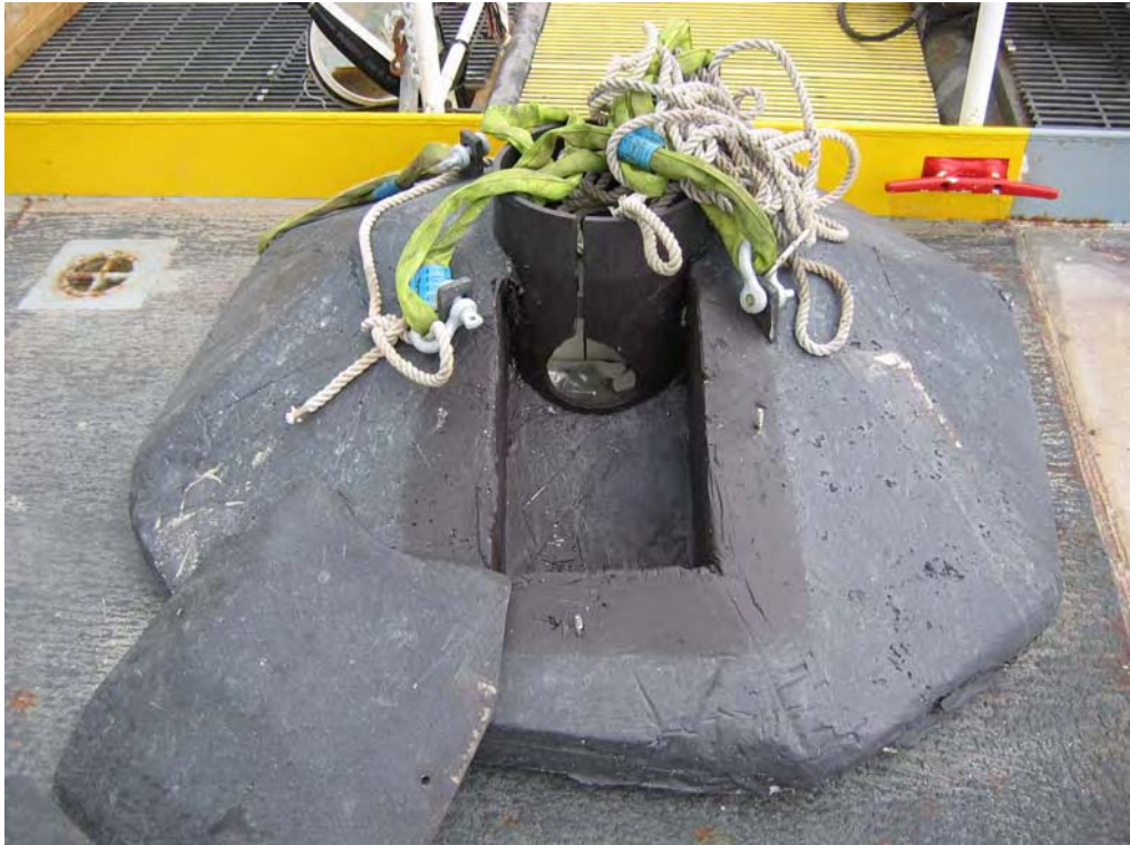
Figure 2: Jacksonville ODMDS Concrete ADCP Base
