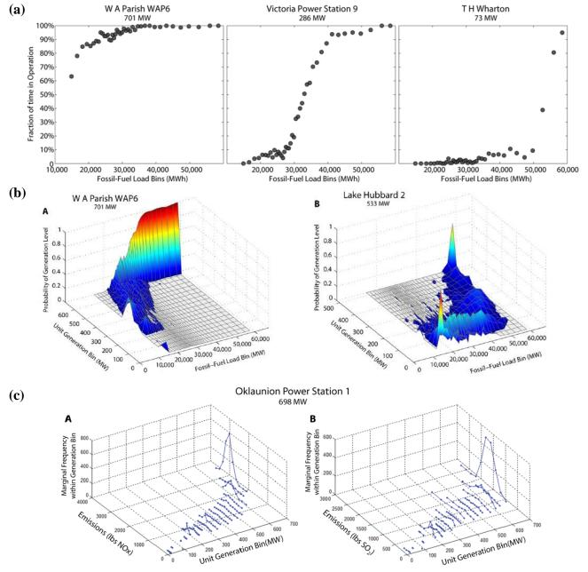
Figure 3. AVERT's statistical algorithm: (a) determine fraction of time units are online, (b) determine generation of units at different load requirements, (c) determine emissions level at generation output
