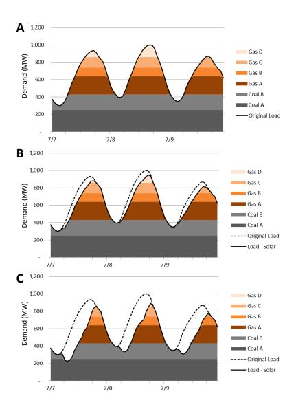
Figure 1. Simplified example of system dispatch over a three day period, and avoided generation from a solar program. (A) Base case; (B) 200 MW solar; (C) 600 MW solar.
