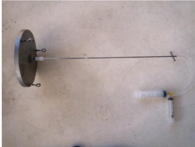
Figure 3: Push Point Pore Water Sampling Apparatus
