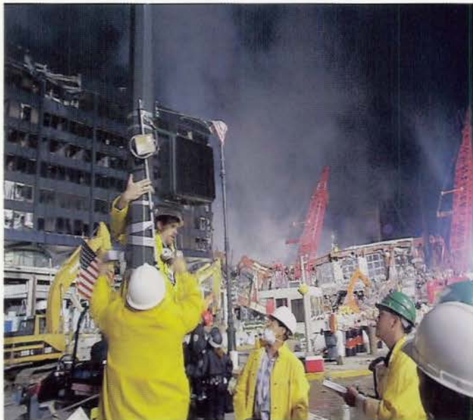
EPA personnel set up an air monitoring station near "ground zero" of the World Trade Center (EPA photo)
