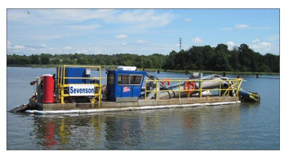
Figure 7. Mud Cat<sup>TM</sup> hydraulic dredge
