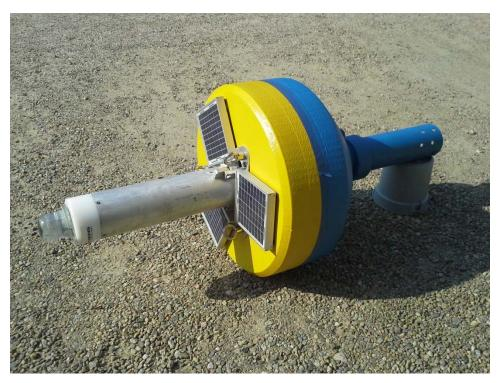
Figure 6. Remote Monitoring Telemetry System Buoy.
