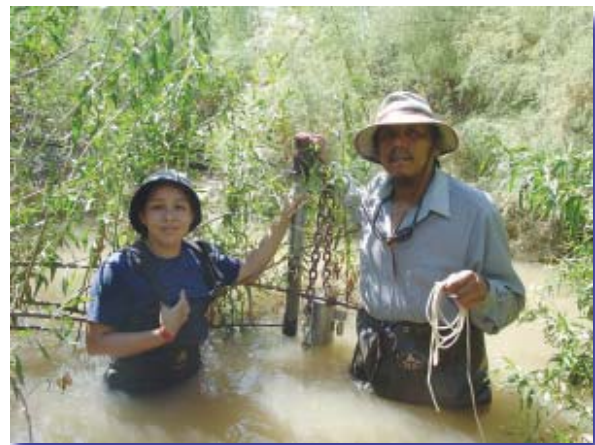
YSI sonde installation for continuous water quality monitoring at the PeePosh Wetlands.
