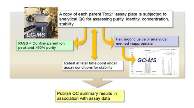
Figure 7. General analytical QC approach for analysis of Tox21 plates.
