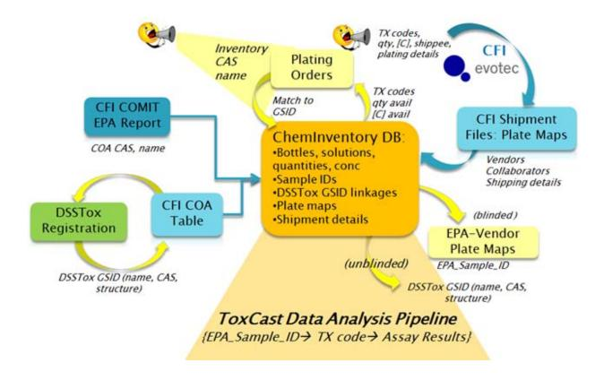
Figure 6. EPA's chemical management processes centrally linked to ChemInventory DB.
