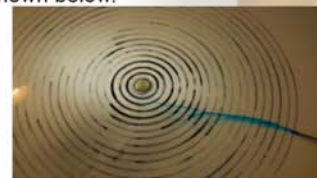
Tracer test during draining of a tank designed to study sediment removal and resuspension. Small changes in design have great impact.
