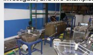
Pilot-scale facility for contaminant fate through waste water treatment, especially activated sludge, systems
