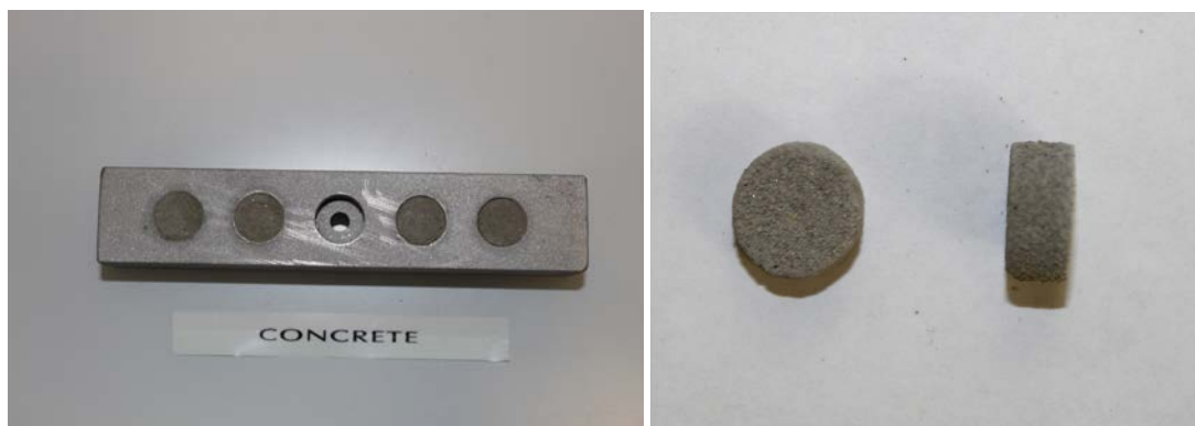
Figure 2.12. Concrete pieces (left: in the stainless steel mold; right: individual coupons)
