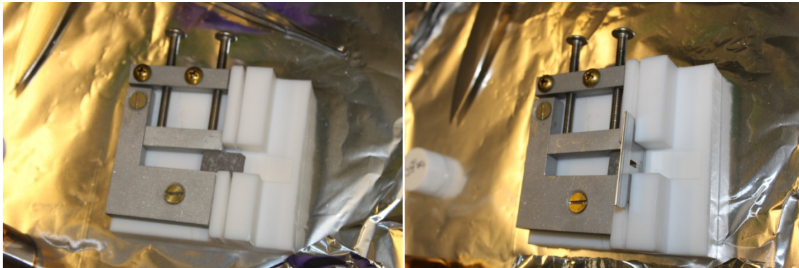
Figure 2.8. Caulk being cut into slices for extraction
