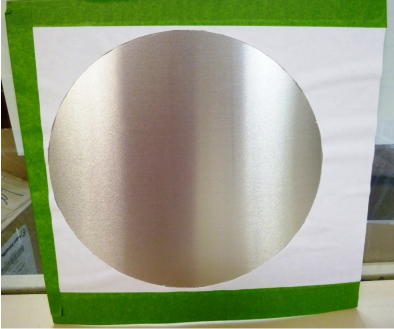
Figure 4.15. Aluminum sheet covered by white shipping label with a 21-cm circle cutout
