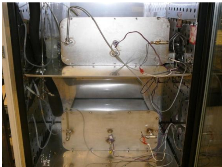
Figure 2.7. Two small environmental chambers in the temperature-controlled incubator
