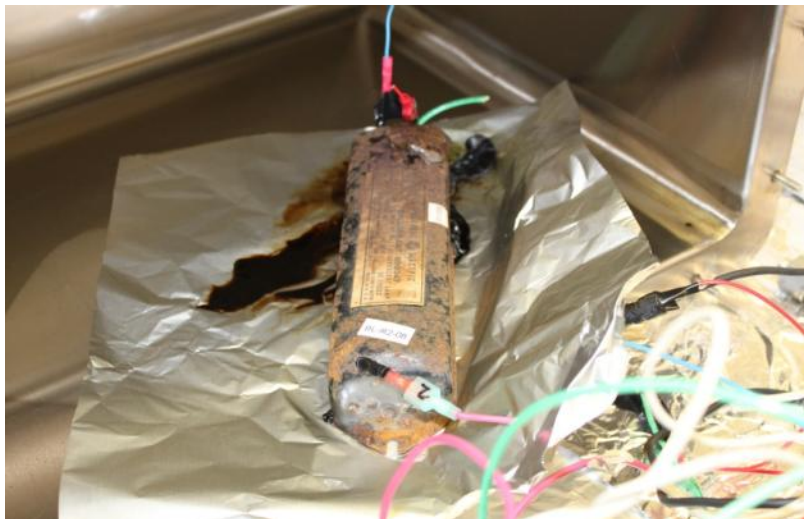
Figure 4.23. Light ballast CK-08 after the burst (the tar-like material is on the right and the gel-like material is on the left)
