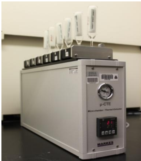
Figure 2.5. Markes \mu -CTE system with polyurethane foam (PUF) sampling tubes
