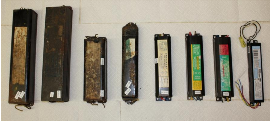
Figure E.5. Part of the light ballasts tested; for comparison, a modern light ballast, marked “PCB-free”, is shown on the far right
