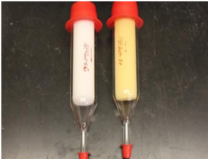
Figure 4.20. Comparison of the PUF sampling cartridge for ballast BL-08 (right) to a normal cartridge (left)
