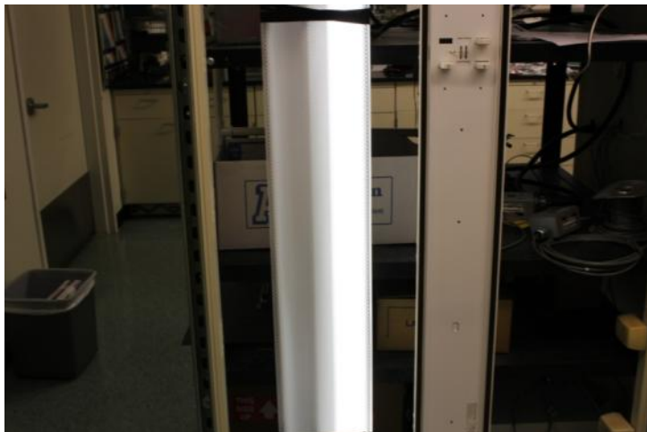
Figure 2.14. Lamp was powered on by the ballast in the chamber
