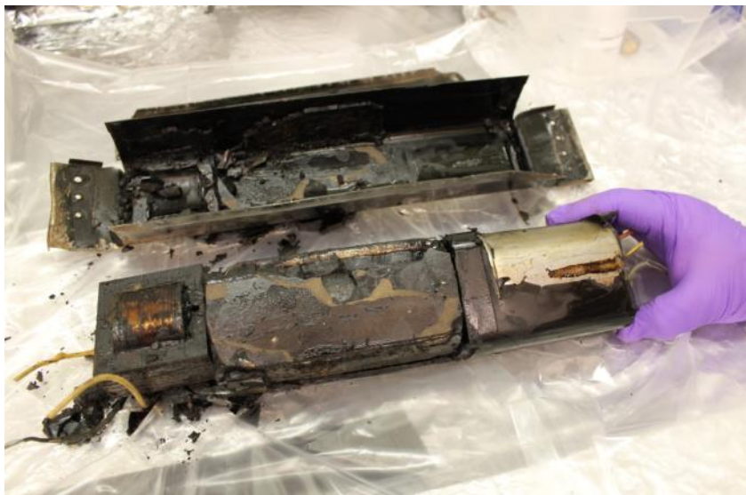
Figure 4.25. Ballast BL-02 (top side) (the capacitor is on the right)
