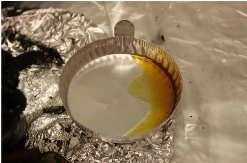
Figure 4.31. Fluid collected from the ruptured capacitor in ballast BL-08
