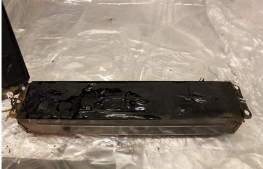
Figure 4.24. Ballast BL-02 after the bottom metal plate was removed (the entire casing was filled with the potting material)
