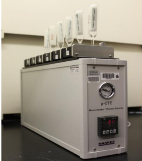
Figure E.1. The micro chamber system with air sampling cartridges
