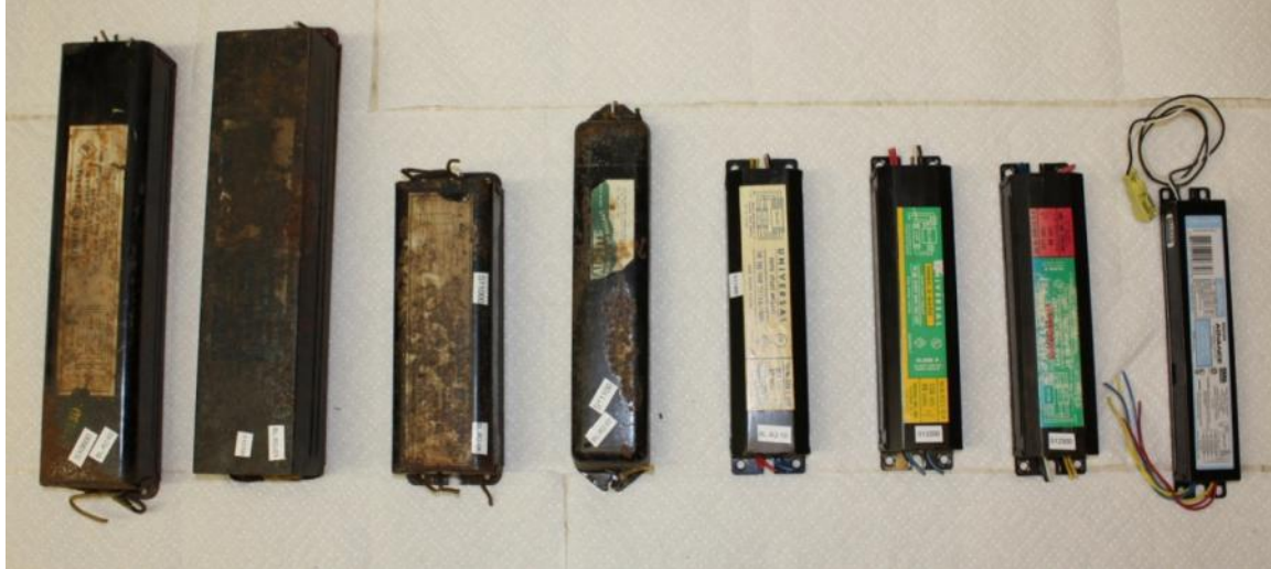
Figure 2.4. Seven of the light ballast samples tested; for comparison, a modern light ballast (marked “PCB-free”) is shown on the far right
