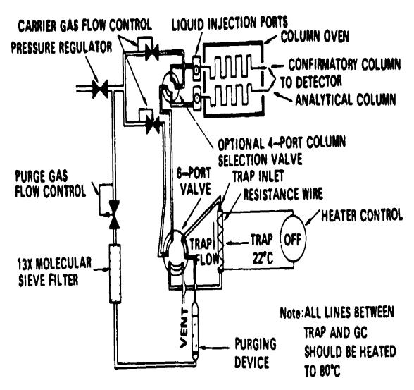
Figure 3. Purge and trap system-purge mode.
