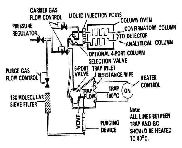
Figure 4. Purge and trap system - desorb mode.
