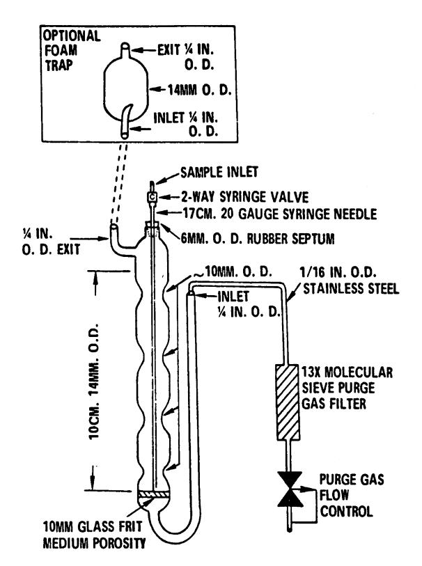
Figure 1. Purging device.
