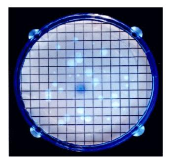
This photograph shows *Escherichia coli* (blue/green fluorescence) and total coliforms other than *E. coli* (blue/white fluorescence) on MI agar under longwave UV light (366 nm). The sample used was a wastewater-spiked Cincinnati, Ohio tap water.
