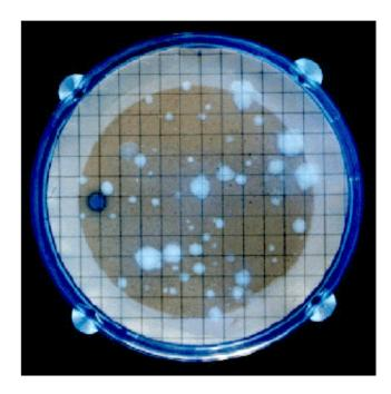
This photograph shows that *Escherichia coli* (blue/green fluorescence) and total coliforms other than *E. coli* (blue/white fluorescence) can easily be detected on MI agar plates from samples with high turbidity levels. The sample used was surface waterspiked Cincinnati, Ohio tap water.
