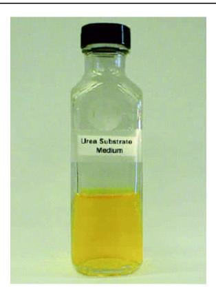
**Photo 1.** Urea substrate medium. After adjusting the pH of the medium to  $5 \pm 0.2$ , the urea substrate medium should be straw-yellow in color.
