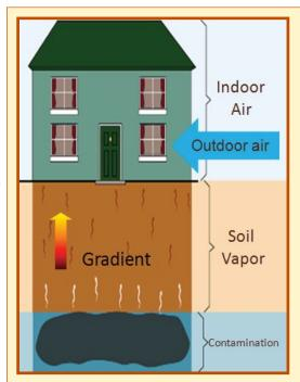
**Figure 1:** "Vapor intrusion" is the movement of chemicals in the soil or groundwater that become a gas easily and can travel into the indoor air of overlying buildings. These chemicals include those called volatile organic compounds (VOCs), such as trichloroethylene (TCE) which is a contaminant at the Grenada site.
