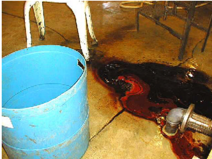
Figure 4. Blood Being Allowed to Flow Directly Into a Floor Drain
