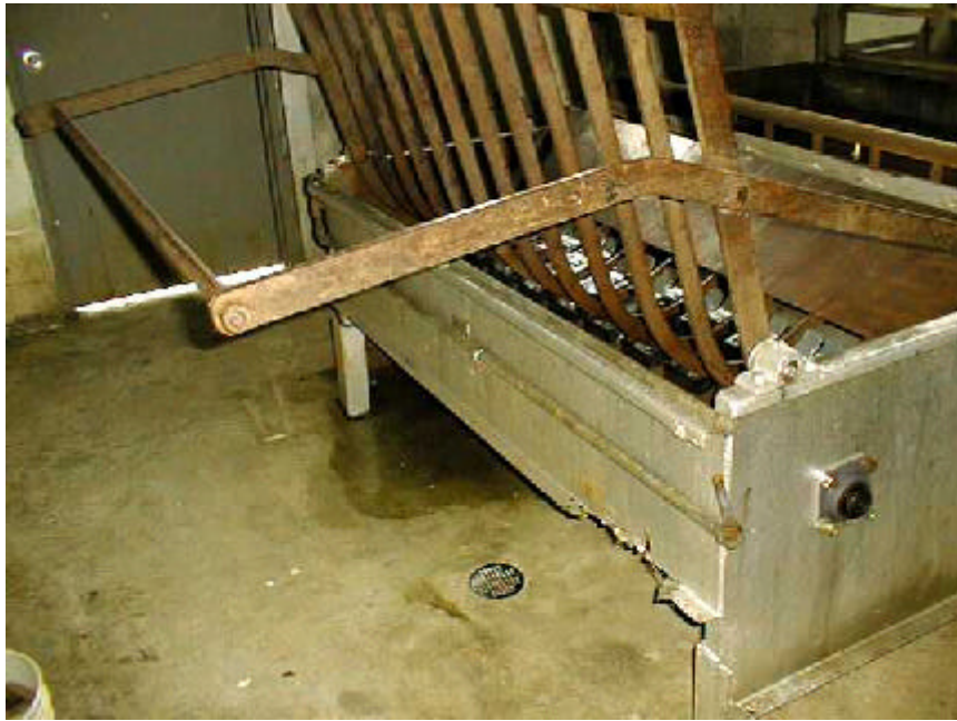
Figure 5. Hog Scalding Machine and Floor Drain
