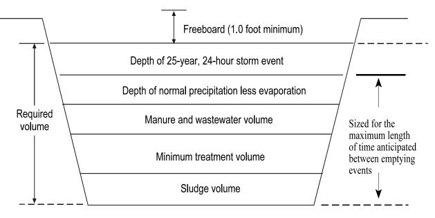
Figure 2-2. Cross Section of Properly Designed Lagoon
