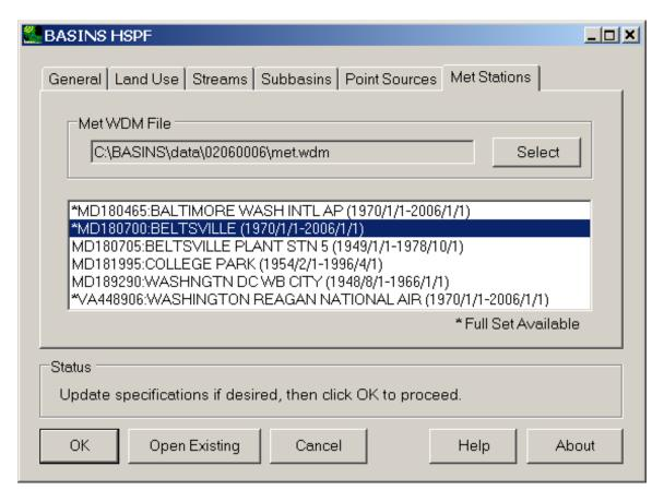
If a station is selected that does not have the full suite, WinHSPF allows the user to specify where to get other needed constituents. For details on the model setup plug-in and WinHSPF working with the meteorological database, see the BASINS User's Manual.
