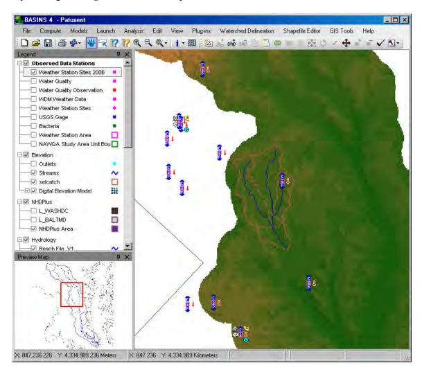
After downloading is complete, a new GIS layer ("Weather Station Sites 2006") is added showing the location of the stations. This layer is stored as a shape file (met.shp) in the BASINS project directory.
