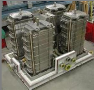
Four-Stack Module 1.4 megawatts
