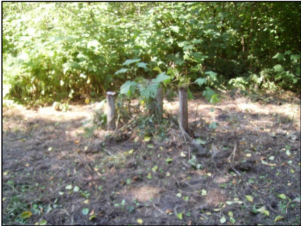
PHOTO 28: Apparent groundwater monitoring well and two bumper posts along bluff.
