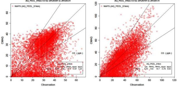
Figure 16c: Scatter Plots of Predicted and Measured Ozone (Left: March; Right: July) AQ\_PEEL\_01km 03 for 20120301 to 20120331 AQ\_PEEL\_01km 03 for 20120701 to 20120731
