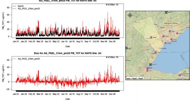
Figure 17a: Timeseries of Predicted and Measured PM<sub>2.5</sub>
